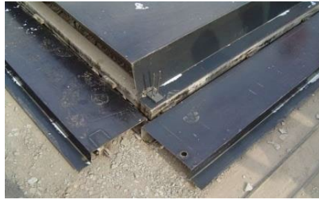
Figure 8: Metal molds for precast concrete elements Source: personal archive of Fabricio (2005).
