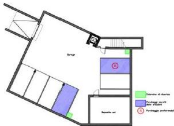
Figure 5: Arrangement of charging station in the basement
