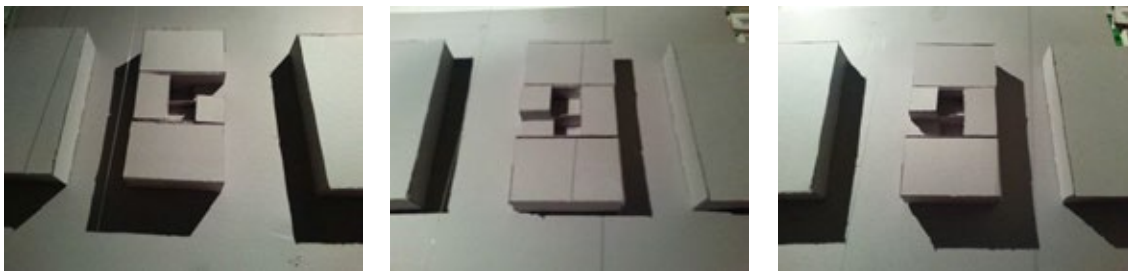
Figure 12: The house project simulation in heliodon in the winter solstice, respectively at 9am, 12am and 3pm Source: Secchin et al. (2013).
