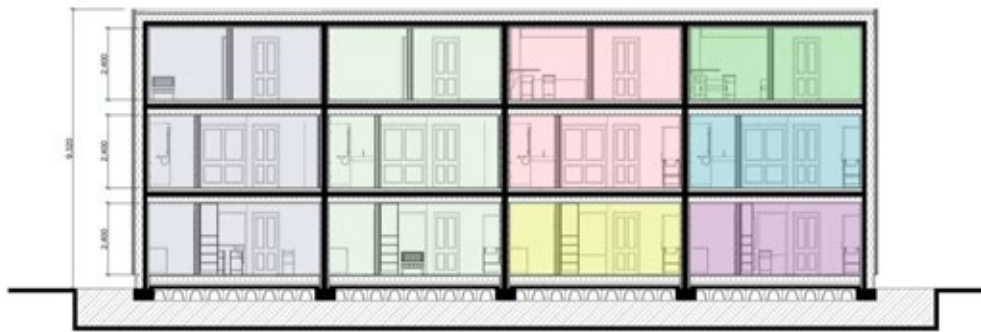
Figure 4: A longitudinal section with growing units
