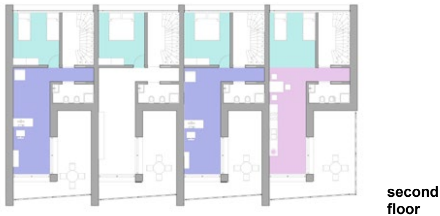
Figure 5: The housing units' floor plans
