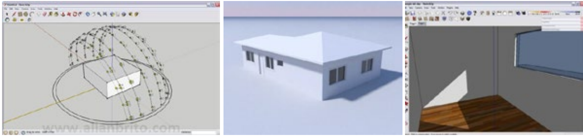
Figure 15: SketchUp® screens showing the virtual heliodon in the software at the left side and studies of external and internal solar incidence on a house project Source: Folha Azero (2008).
