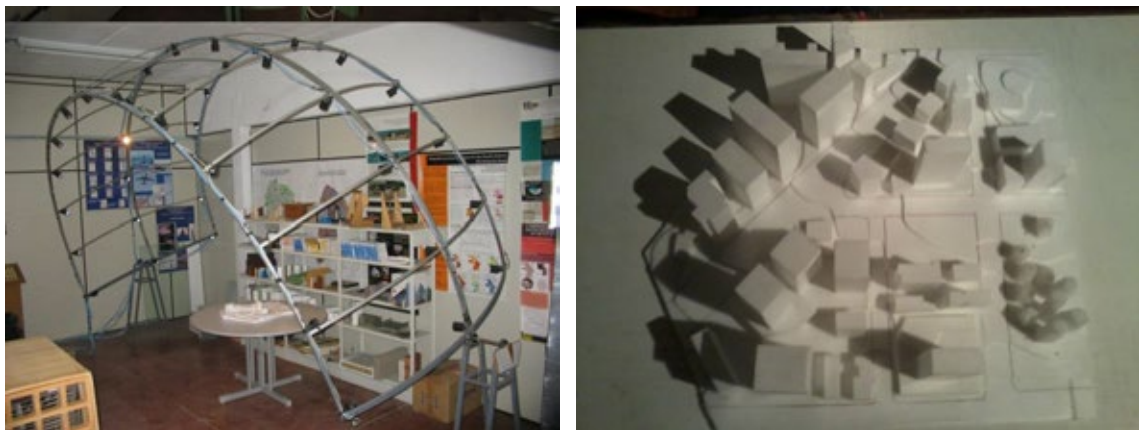
Figure 9: At the left side the heliodon with its three arcs representing the trajectories of the sun in the solstices and equinoxes – each lamp represents a specific hour – at the right side an urban mock-up being tested
