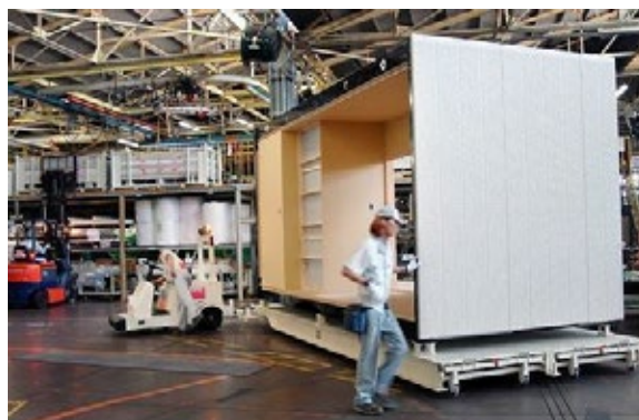
Figure 6: Completed module that will be part of a Toyota housing unit Source: Seattle Times (2014).
