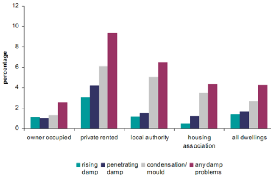
Figure 1: Percentage of houses with damp problems (2012) Source: Department for Communities and Local Government (2014).
