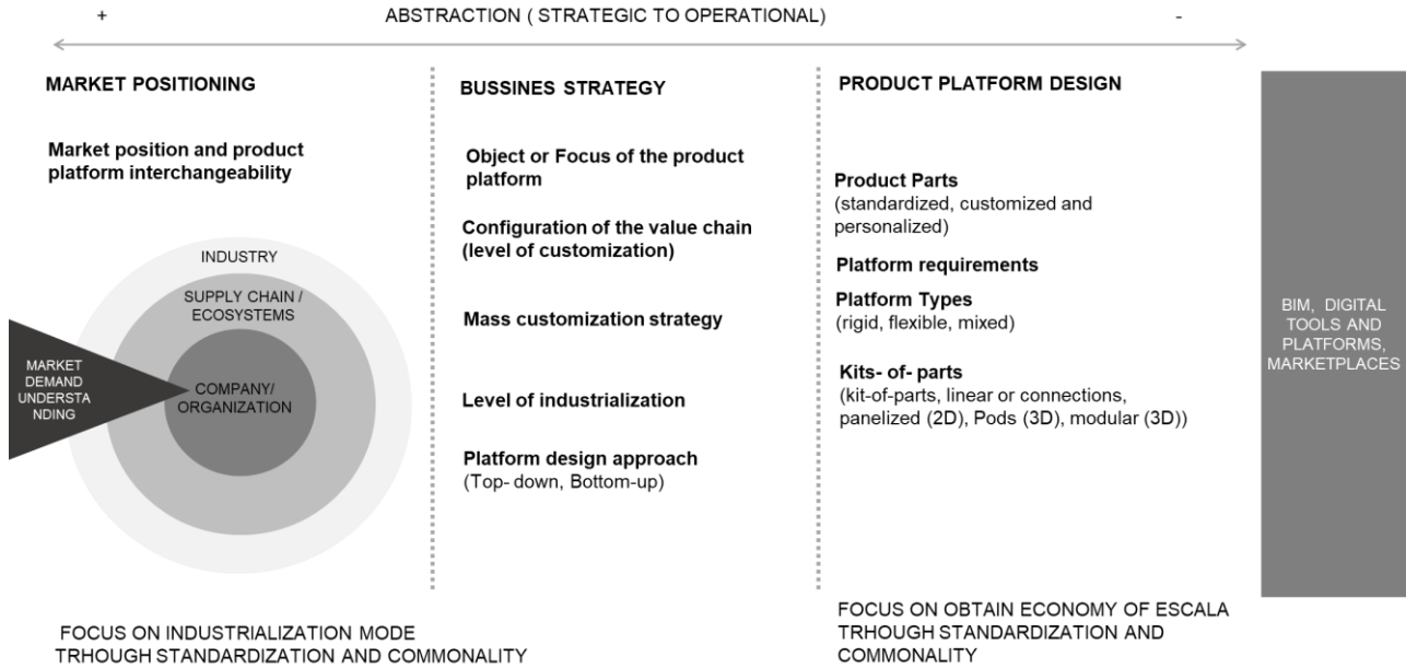
Figure 1: Model for implementing product platforms in construction.
