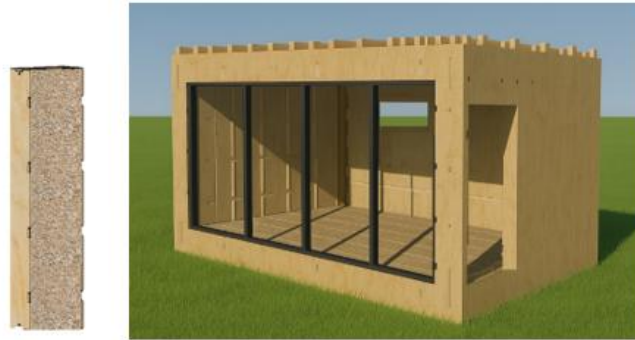
Figure 1: Wikihouse modular prototype and insulated wall section with rice husk infill.
