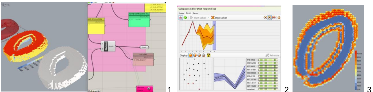
Figure 4: Image for Series-1 : 1. Solar insolation and massing design of cell aggregation 2. Galapagos results for DA % & 3. Middle floor DA% results for cell aggregated of the massing design
